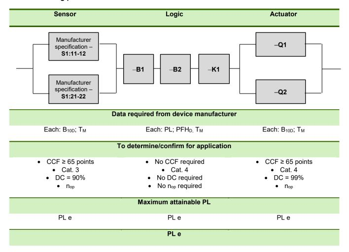
Door switch, RFID & emergency stop in series (2) - emergency stop in PL e
