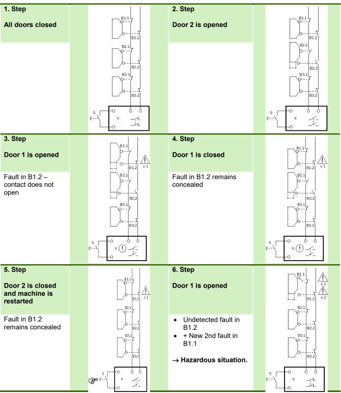
Illustration 5: Direct fault masking per ISO/TR 24119
