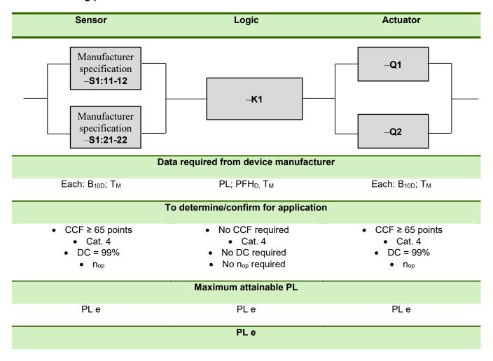
EMERGENCY stop - 2-channel, cross short circuit detection in PL e
