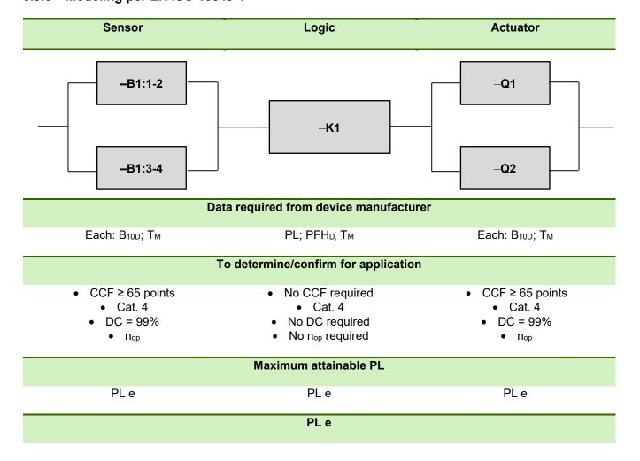
Door switch, magnetic – 2-channel, equivalent in PL e
