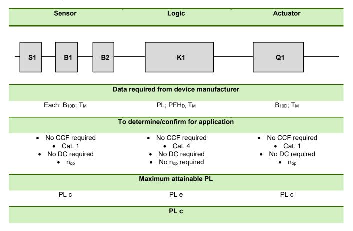
EMERGENCY stop & door switch, magnetic in series, 2-channel in PL c
