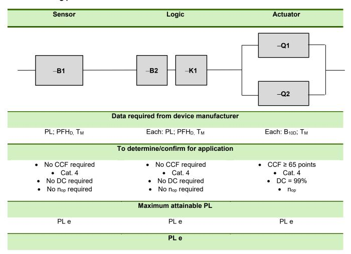
Door switch, RFID & emergency stop in series (1) - door -B1 in PL e
