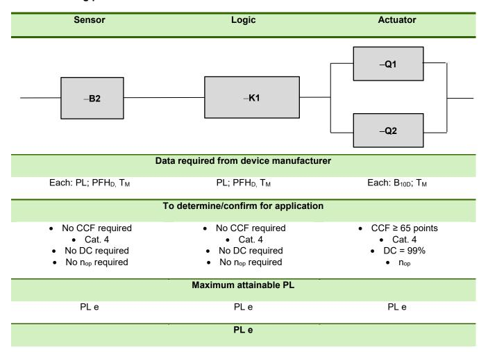
Door switch, RFID & emergency stop in series (1) - door -B2 in PL e
