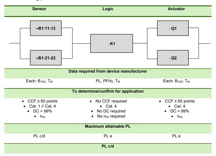
Door switch, mechanical - 2-channel equivalent in PL c/d
