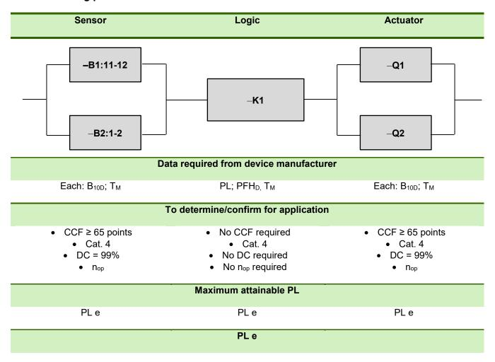
Door switch, mechanical & magnetic - each 1-channel in PL e
