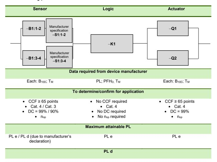
Magnetic door switch and pressure-sensitive mat - cross circuit in PL d
