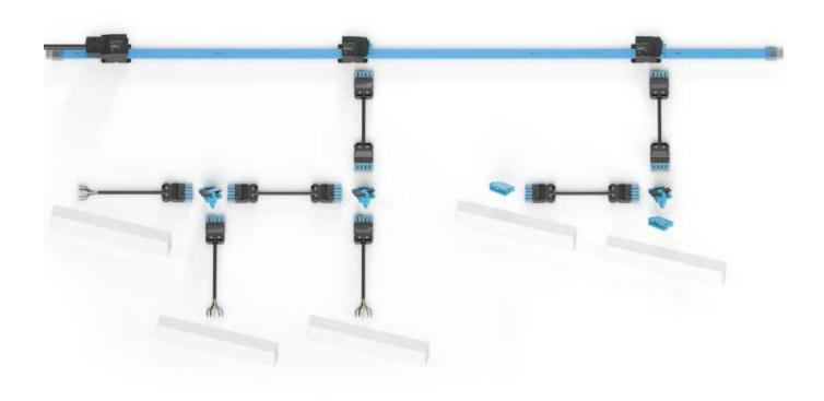
With gesis®NRG in combination with gesis®CLASSIC, it is extremely simple to supply DALI luminaires, for example. This allows a flexible choice of connection technology for the luminaires. With applications over a large area with long cable lengths, a 7-pole gesis®NRG flat cable is also available for combining three-phase current and dimming signal.
