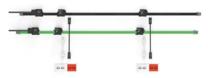
The gesis®NRG flat cables 5G2.5/4 mm<sup>2</sup> can also be used in cable trays thanks to the tap which is routed parallel to the cable. Three-phase power supply up to just before the socket ensures reduced energy consumption. The availability of several cable colors makes it easier to distinguish between networks (NN/IT or general/emergency). The 3-pole, pluggable taps with free phase selection enable flexible load sharing.
