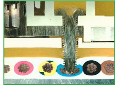
Fig. 1 Cross-section view of the Copper Displacement terminal making contact
