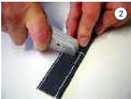
Scratch the flat cable as follows: 1x all around in the transverse direction and then 2x in the longitudinal direction on both sides The longitudinal cut should end shortly before the transverse cut in order to prevent tearing
