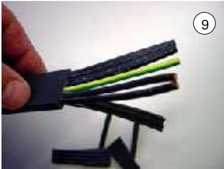
Pull off the web with the remaining sheath residue
